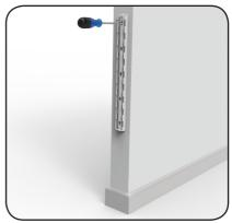
Place the assembled barrier against the wall and mark position. Remove bracket from cover and hold in marked location, and mark screw positions.Screw into surface with the appropriate fixing method.
