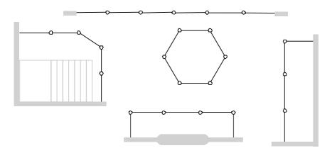
Up to 6 panels including the gate may be used in open configurations providing the 2 end panels are securely fixed to a wall with the fixings provided.
